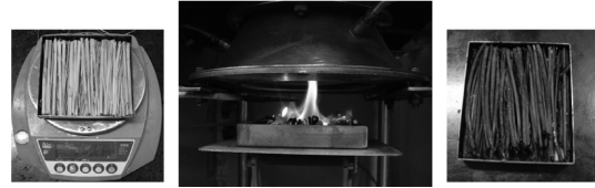
Figure 2. Photograph of combustion test by cone heater.
