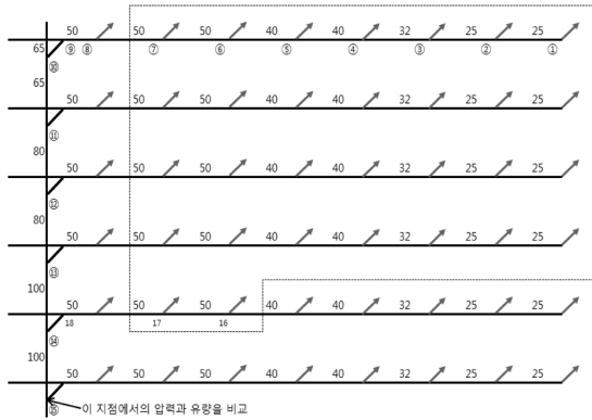
Figure 5. Case of 1.2 times longer of branch side (Demand of NFPA 13).
