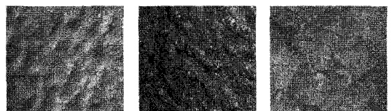
(a) 1.0 ~ 1.5 mm (b) 0.75 ~ 1.0 mm (c) 0.5 ~ 0.75 mm Fig. 10 Damaged surfaces (nozzle feed: 5 mm/s, nozzle pressure: 0.45 MPa)
