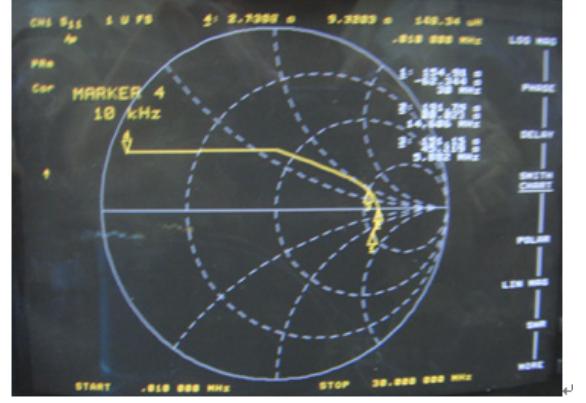
Fig. 3 Test results of S-parameter (S11) of unmatched Coupler
