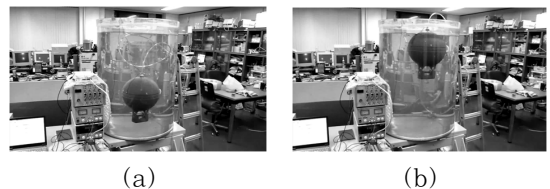
Figure 7: Submersible buoy during sinking(a) and floating(b) by automatic control system
