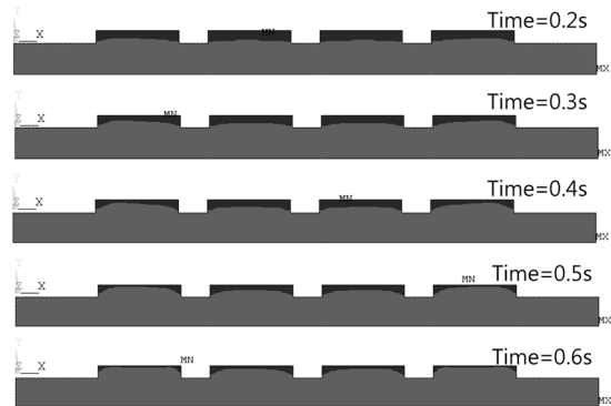
Fig. 4. Free surface shapes at time passing under the conditions of V = 2 \text{ mm/s} .
