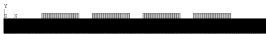
Fig. 3. FEM model in initial condition where gray elements correspond to resist flow, and the white elements relate to air.
