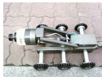
(b) CCTV for pipe inspection
