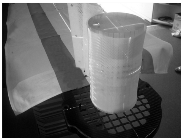
Fig. 5. With the immobilization mask, the surface doses were measured by placing the TLDs on the surface of a cylindrical phantom in each 10° angular position.
