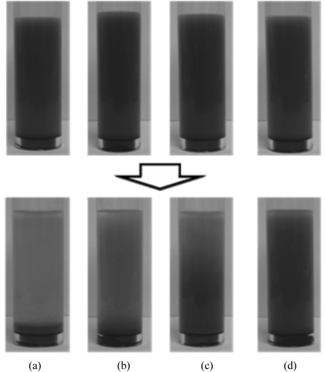
Figure 6. Sedimentation of the treated ATO solutions after 1 h; (a) BM0-ATO, (b) BM20-ATO, (c) BM40-ATO, and (d) BM60-ATO.
