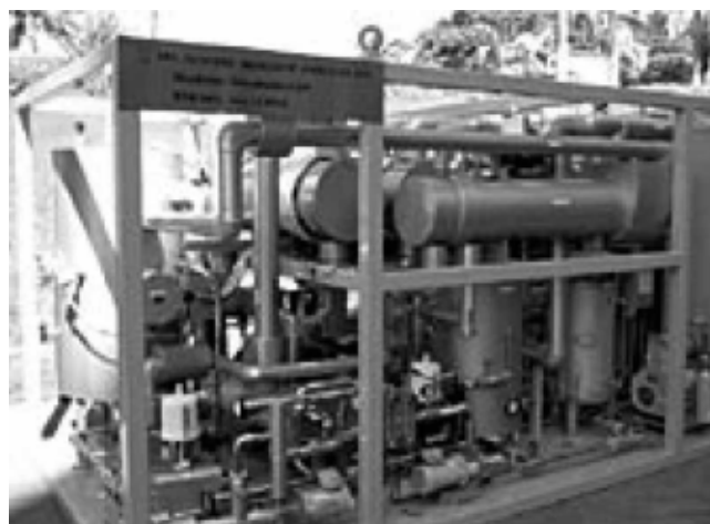
Figure 4. A-type zeolite membranes for dehydration of bio-ethanol commercialized by Mitsui ( www. mitsui.co.jp ).
