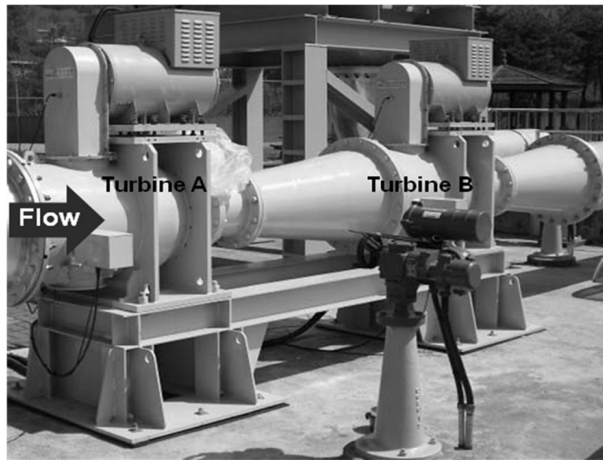
Fig. 4 Serial arrangement of two tubular turbines for field test
