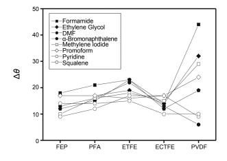
**Figure 4.** Contact angle hysteresis of the probe liquids on the fluoropolymers: formamide (filled squares), ethylene glycol (filled diamonds), DMF (filled circles),  $\alpha$ -bromonaphthalene (filled pentagons), methylene iodide (hollow squares), bromoform (hollow diamonds), pyridine (hollow circles), and squalene (hollow pentagons).
