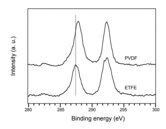
Figure 2. XPS spectra of the  $C_{1s}$  region for ETFE and PVDF.
