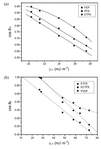
**Figure 3.** Zisman plots of  $\cos\theta_a vs. \gamma_{LV}$  for various probe liquids on selected fluorinated polymers. (a) Nonpolar aprotic liquids: heptane, octane, decane, tridecane, and hexadecane on FEP, PFA, and ETFE. (b) Polar protic liquids: water, formamide, glycerol, ethylene glycol, decanol, and heptanol on ETFE, ECTFE, and PVDF.
