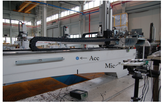
Fig. 5 Photograph of the noise experiment for the take-out robot
