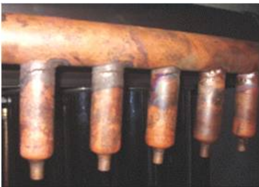
Fig. 2 Manifold in vacuum tube type solar collector
