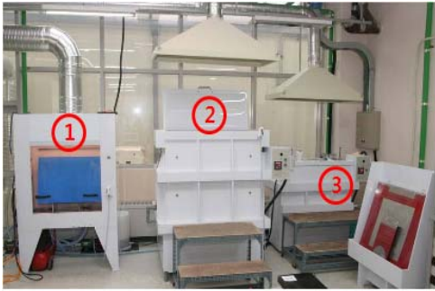
Fig. 3 A photograph of electroforming machine: silver spray booth, ② electroforming bath, ③ cleaning bath
