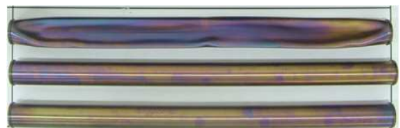
Fig. 2 Typical view of collapsed and non-collapsed tube specimen (at pressure difference of 3.893 MPa)
