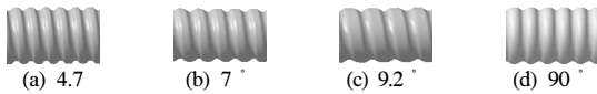
Fig. 3. Inclined angle models for a corrugated flexible pipe with a same corrugation height of h=1.5mm.
