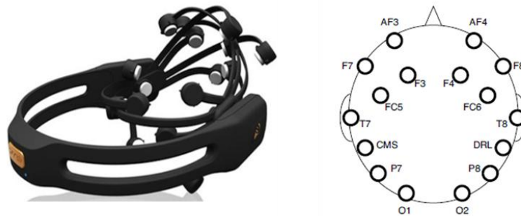
Fig. 3. Epoc neuro-headset (right) and its electrode location(left)
