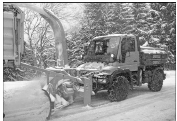
Figure 7. Snow transfer by blower(www.schmidt.com)
