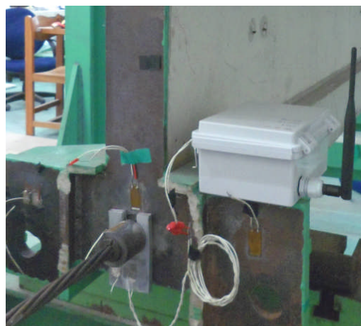
Fig. 5 Experimental setup on tendon-anchorage connection of prestressed concrete girder
