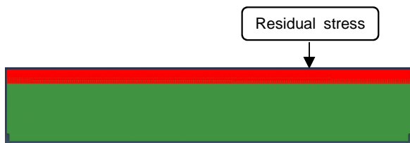
Fig. 5 The setup of different depth of residual stress layer (16 meshed layers of top surface) for the modeling
