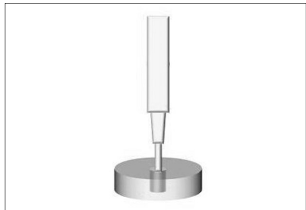
Figure 2. 2-Schematic drawing of push-out strength test.
