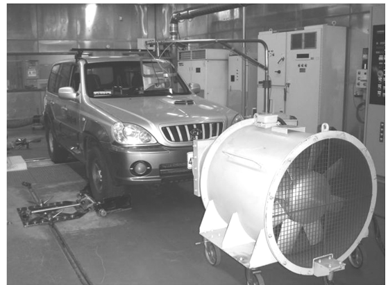
Fig. 1 Experimental setup of chassis dynamometer test for vehicle emission measurement
