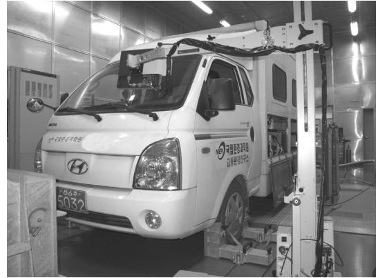
(a) Test vehicle on chassis dynamometer
