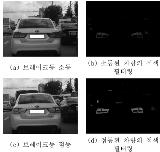
Fig. 1. Brake lights of a white vehicle turned on/off, and its respective R-filtered images.
