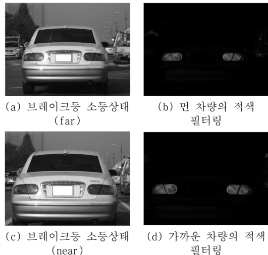
Fig. 5. Vehicle approached with brake lights turned off, and its respective R-filtered images.
