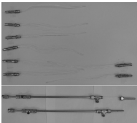
Fig. 6. Photograph of the test module for hollow fiber membrane and housing.
