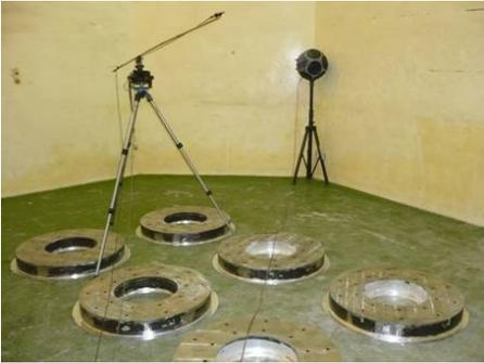
Fig. 4 Measurement of random incidence absorption coefficient in a reverberation room
