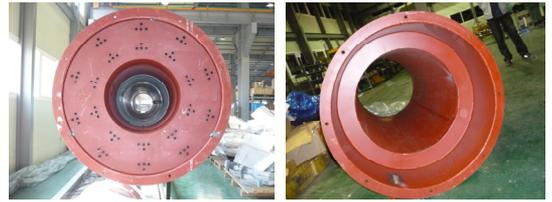
Fig. 8 Ring-shaped resonator installed in test silencer
