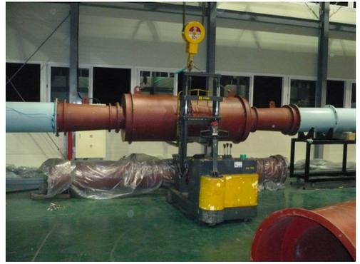
Fig. 7 Insertion loss test for silencer with ring-shaped resonator
