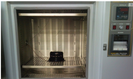
Figure 8: Low temp. fire test set-up
