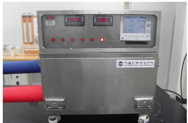
Fig. 2 In-Situ ground effective thermal conductivity test unit.
