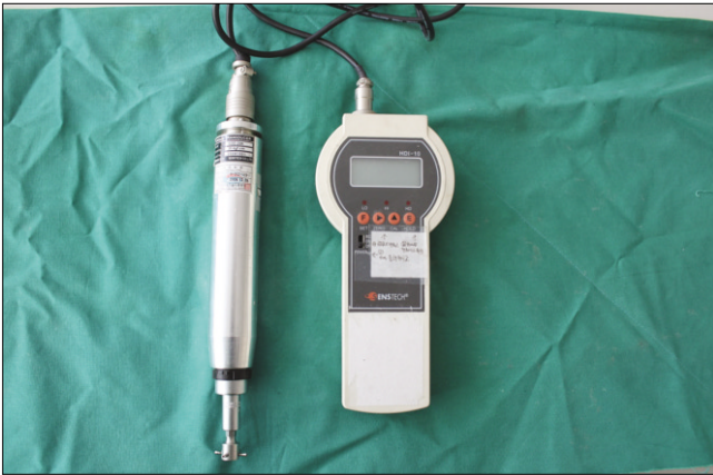
Fig. 1. Digital torque meter used to measure the peak value of resistance to reverse torque rotation in N cm.
