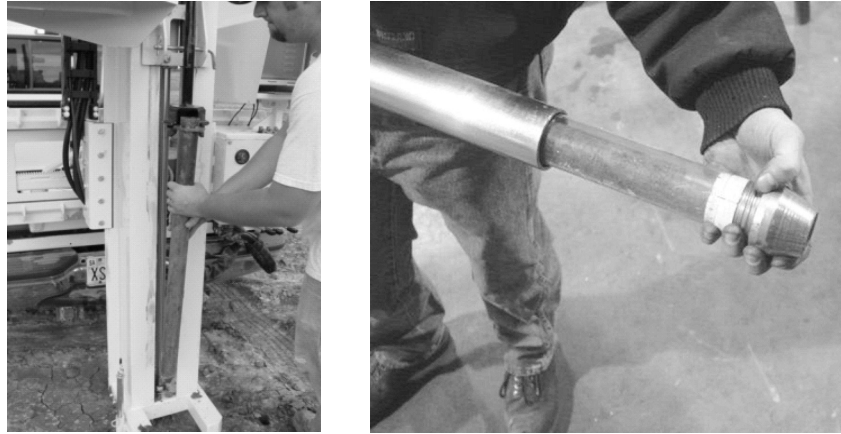
Fig. 2 A soil core extracted using a Veris Technologies hydraulic probe unit.
