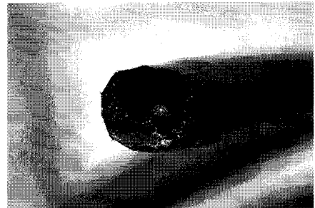
(c) Snapped power cable of the distribution line
