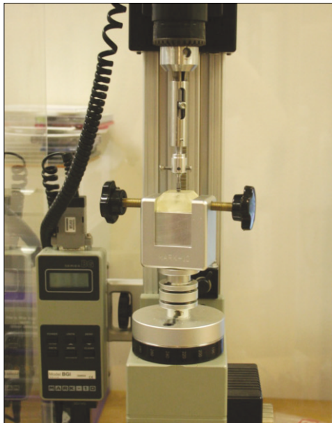
Fig. 6. Removal torque test with motorized torque test stands, TSTM.
