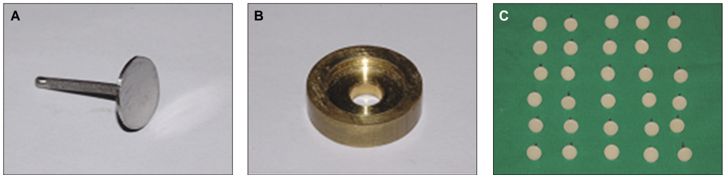
Fig. 3. Procedure of specimen fabrication. A: Metal coping, B: Mold for porcelain build up, C: fabricated specimens.
