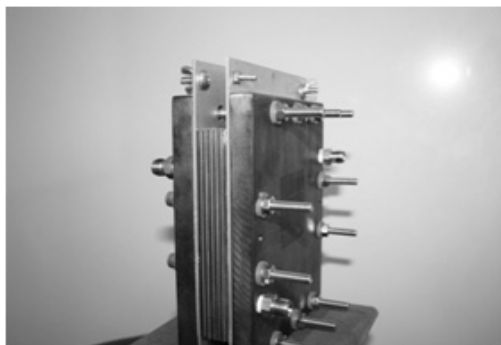
Fig. 1 Photograph of the direct methanol fuel cell composed of five stacks
