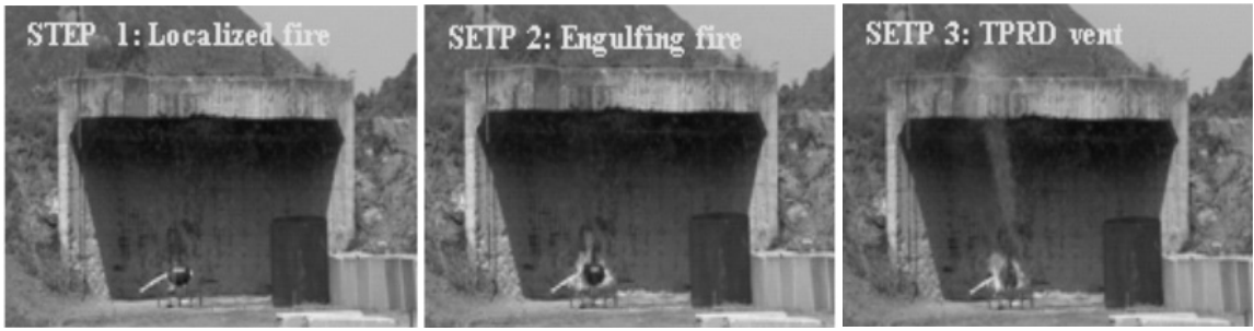
Fig. 7 Fire status of the hydrogen tank for step
