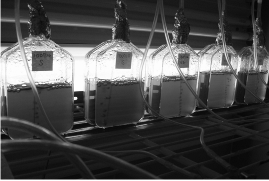
Fig. 2 Experimental setting for synchronization of cyanobacterial cultures
