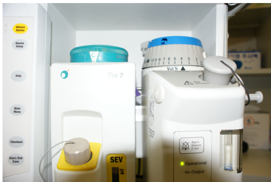
Fig. 1. The vaporizer can be turned “ON” when the mismatched locking lever is maintained at the “Lock” position. The vaporizer on the left is Sevoflurane and the one on the right is Desflurane.
