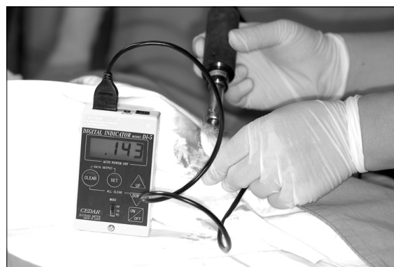
Fig 3. The digital torque gauge used in this study.
