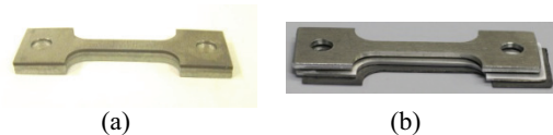
Fig. 2 Tensile specimens of multilayered sheet and separated sheet: (a) multilayered sheet, (b) separated sheet
