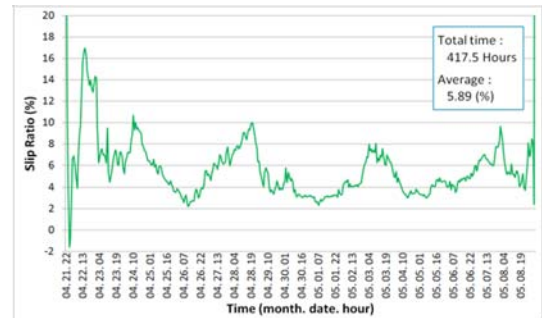
Figure 17: Ship slip ratio from Kaohsiung port to Panama Canal
