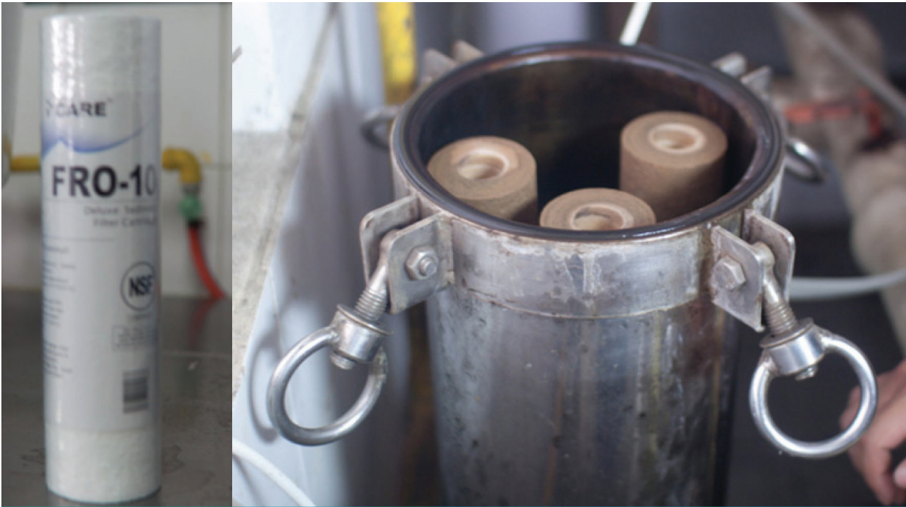
Figure 4. Unused underground water filter (left, white color); Used underground water filter (right, dark-brown color).
