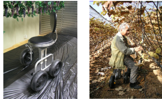
Figure 2. Working chair for grapevine cluster thinning [(a) laboratory, (b) field in grapevine yard]
