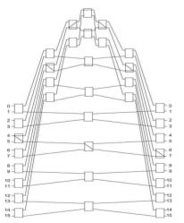
[Fig. 6] Alternative paths for fault tolerant in 16×16
