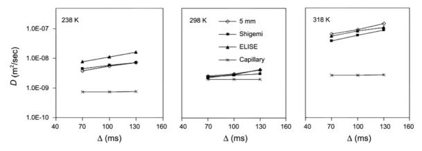
**Figure 3.** Comparison of the measured diffusion coefficients (*D*) of chloroform at 238 K, 298 K and 318 K with varying diffusion time ( $\Delta$ ). The graphs correspond to the data in Table 1.
