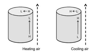
**Figure 2.** Variations of temperature gradients expected when hot or cold air is supplied from the bottom of the NMR tube, where H and L represent the high- and low-temperature components induced by the air flows, respectively.
