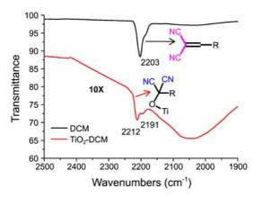
Figure 3. FTIR spectra of DCM and DCM/TiO<sub>2</sub>.
