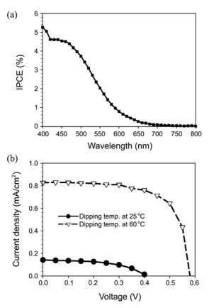
Figure 5. (a) IPCE curve of DCM-sensitized DSSC. (b) Photocurrent action spectra of DCM-sensitized solar cells using liquid iodide electrolytes.
