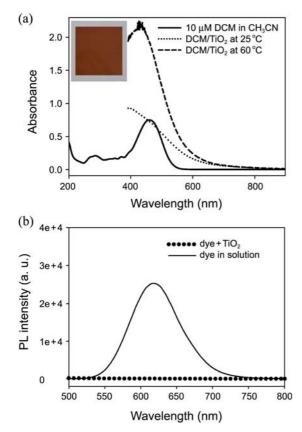
**Figure 4.** Absorption (a) and fluorescence (b) spectra of DCM in acetonitrile and DCM/TiO<sub>2</sub>.
