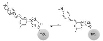
Figure 2. Molecular structure of DCM binding to the titania surface.
