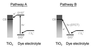
Figure 1. Two different electron injection models from adsorbed dyes into  $TiO_2$  conduction band.
