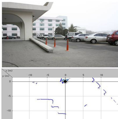
Figure 5. Performance test of LMS151(1)
