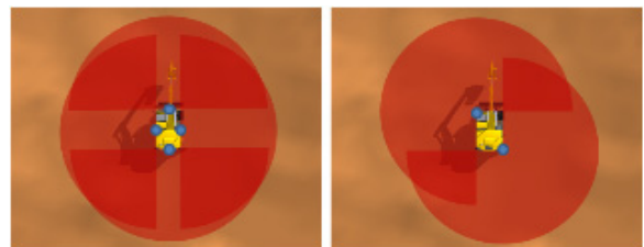
(a) Object detection area(LMS221) (b) Object detection area(LMS151)
