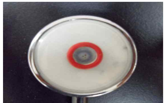
Fig. 3. The photo of pulse sensor using stethoscope
