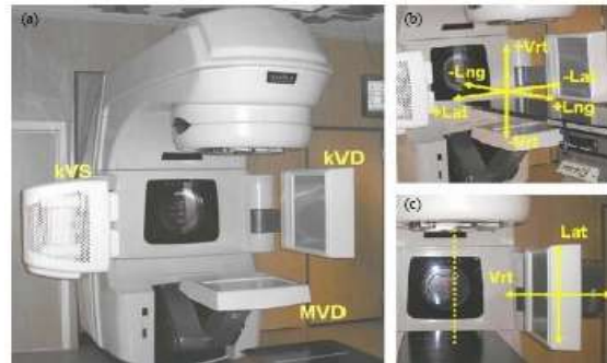
Fig. 1. (a) Varian clinical linear accelerator with an on-board imager® (OBI) consisting of two robotic arms; one holding a flat panel imager (kVD). The mega voltage detector (MVD) is also extracted. (b) The coordinate system for couch/patient position: lateral = + right/-left, vertical=anterior/-posterior and longitudinal =+inferior/-superior. (c) lateral and vertical motion of the kVD are relative the MV beam axis.
