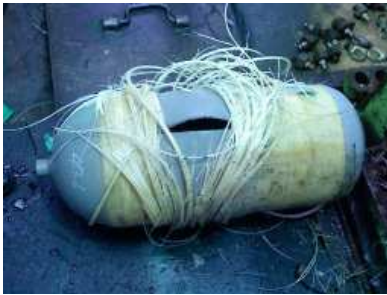
Fig. 4 Fuel tank after burst test
